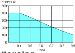
**Note:** Clearance gap F is the maximum permissable. i.e. gap completely on one side, in the temperature range of  $-30^{\circ}$ C to  $80^{\circ}$ C
