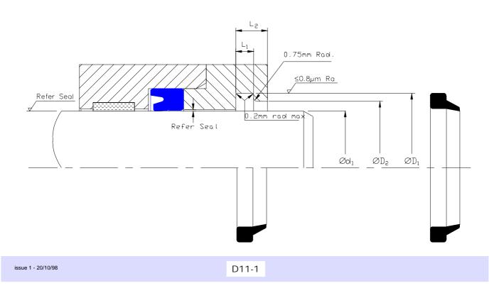
ClaronPolyseal® Single Acting Rod Wiper Seal
